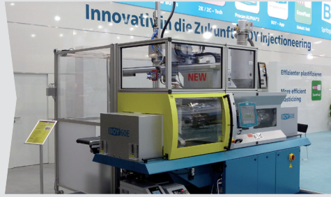
Production cell with CE-compliant safety housing
